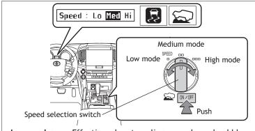
**Low mode:** Effective when traveling on rocks and pebbles. **Medium mode:** Effective when traveling on snow or descending a
